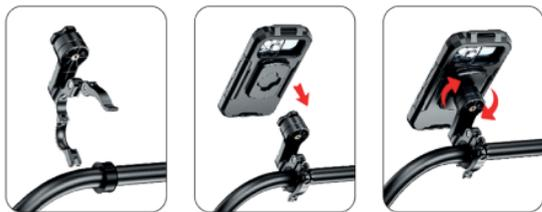
.1 Open the quick-release buckle and install it in the appropriate position.
