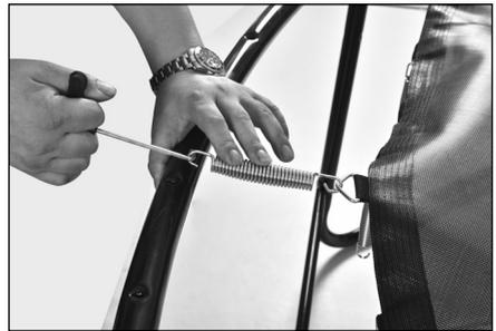
8. Repeat the process for all springs (H). Use the springs mounting tool (I).
